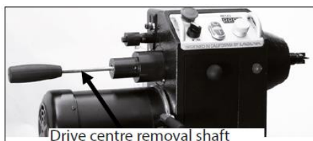
Drive center removal shaft
